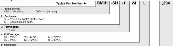
D = Standard (720mW) L = Sensitive (540mW)
