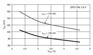
**Dropout Voltage vs. Output Voltage**
