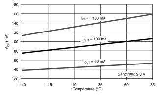
**Dropout Voltage vs. Temperature**
