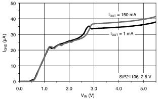
Ground Current vs. Input Voltage at 25 °C
