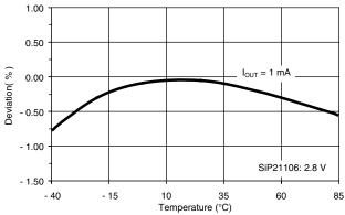
**Output Voltage Accuracy vs. Temperature**
