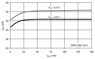
**Ground Current vs. Output Current**
