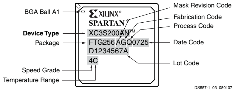
Figure 4: Spartan-3AN FPGA BGA Package Marking Example
