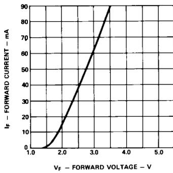
Figure 2. Forward current vs. forward voltage characteristics.
