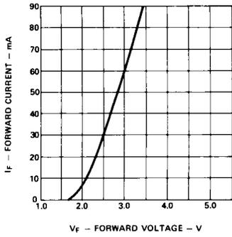
Figure 12. Forward current vs. forward voltage characteristics.
