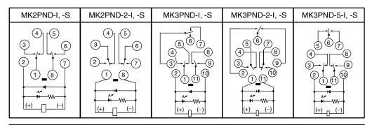
**LED Indicator and** Varistor Type (AC Coil)
