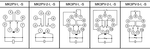
**LED Indicator and Diode Type** (DC Coil)
