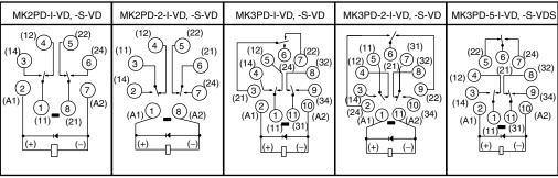
VDE Approved Type Diode Type (DC Coil: Reverse Polarity)
