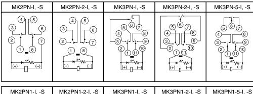
Diode Type (DC Coil: Standard Polarity)
