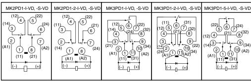
VDE Approved Type LED Indicator Type (AC Coil)
