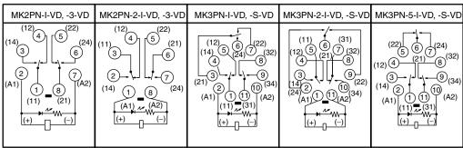
**VDE Approved Type LED Indicator Type** (DC Coil: **Reverse Polarity)**
