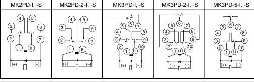
Diode Type (DC Coil: Reverse Polarity)
