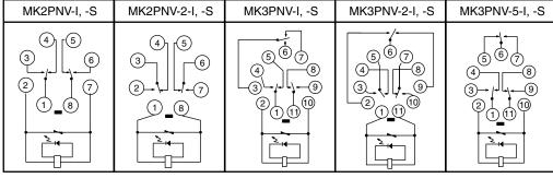
**VDE Approved Type LED Indicator Type** (DC Coil: Standard Polarity) (): Dual Numbering
