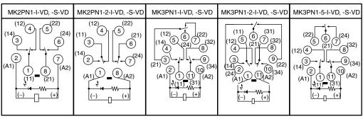
**VDE Approved Type Diode Type** (DC Coil: Standard Polarity)
