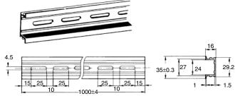
\* A total of twelve 25 x 4.5 elliptic holes is provided with six holes cut from each track end at a pitch of 10 mm.
