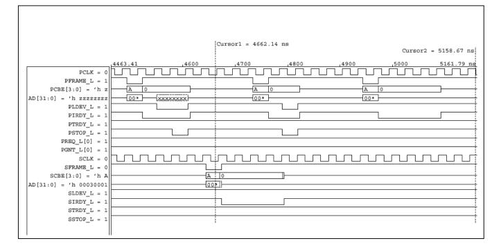
Figure 2 : Primary to Secondary Type 1 to Type 1 Configuration Cycle passing.
