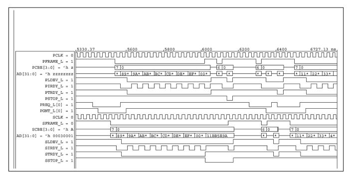
Figure 7 : Secondary to Primary Memory Write transaction.
