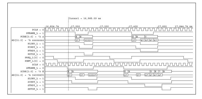
Figure 3 : Secondary to Primary Memory Read Line transaction.
