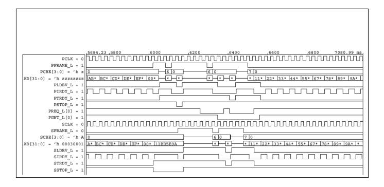
Figure 4 : Primary to Secondary Memory Read transaction.
