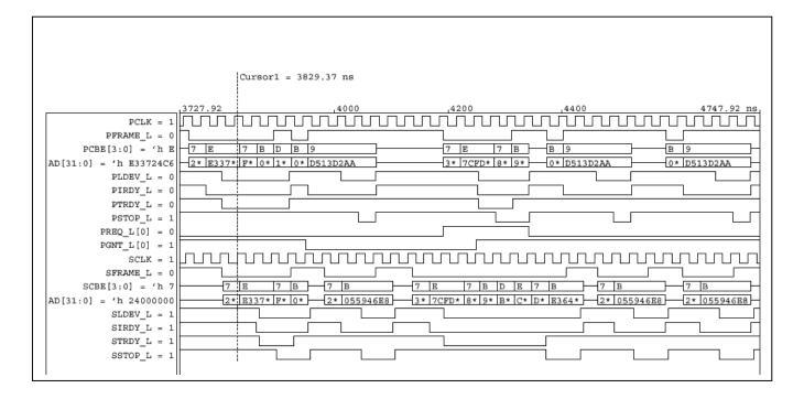
Figure 6 : Primary to Secondary Memory Write transaction followed by Secondary to Primary Memory Write transaction.
