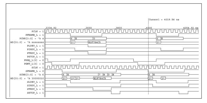
Figure 5 : Secondary to Primary Memory Read transaction.
