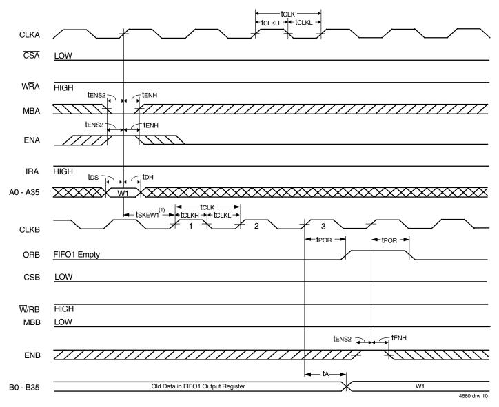
Figure 8. ORB Flag Timing and First Data Word Fall Through when FIFO1 is Empty
