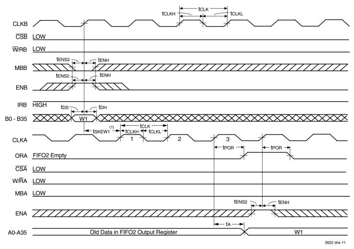
Figure 9. ORA Flag Timing and First Data Word Fall Through when FIFO2 is Empty
