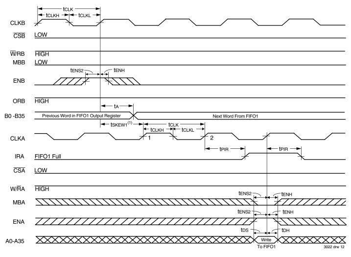
Figure 10. IRA Flag Timing and First Available Write when FIFO1 is Full
