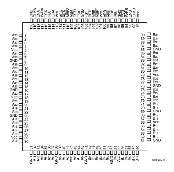
TQFP (PN120-1, order code: PF) TOP VIEW
