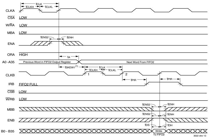
Figure 11. IRB Flag Timing and First Available Write when FIFO2 is Full
