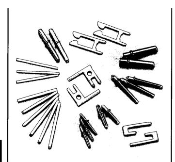
Various pins and wrap posts are available. The tips of the RT pins and the wrap posts are pyramid shaped to ensure smooth insertion into printed circuit boards. The RT pins are perfectly round since they are formed by drawing. The square wrap post is smooth on four sides but has sharp corners to ensure a secure and reliable wrapped connection.
