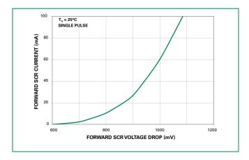
Figure 3: High Current SCR Forward Voltage Drop Curve
