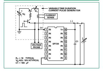
Figure 5: SP720 Typical Nonrepetitive Peak Current
