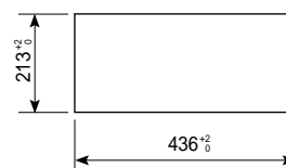
Panel cutout (for flush mounting)
