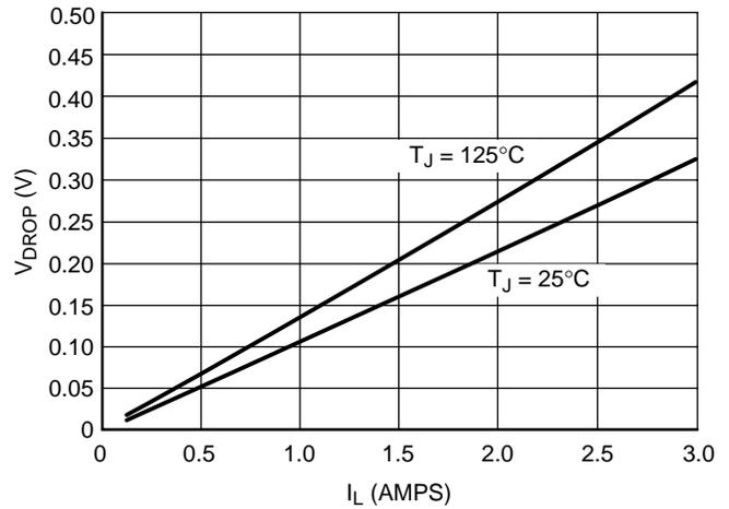
Figure 3.  $V_{\text{drop}}$  vs.  $I_L$  @  $V_{\text{in}} = 4.5 \text{ V}$
