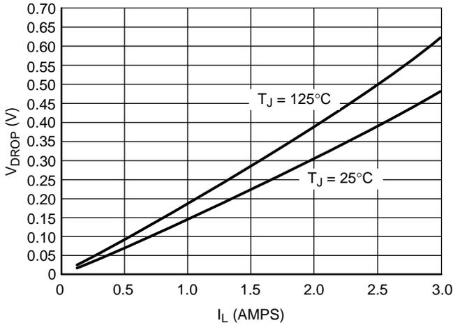
Figure 2.  $V_{\text{drop}}$  vs.  $I_L$  @  $V_{\text{in}} = 2.5 \text{ V}$
