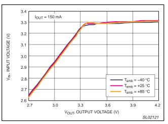
Figure 6. Input voltage versus output voltage.
