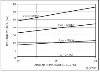
Figure 3. Drop-out voltage versus temperature.
