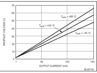
Figure 4. Dropout voltage versus output current.
