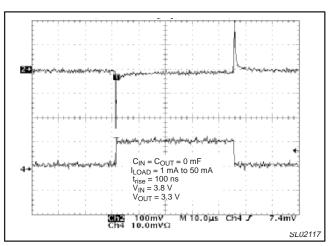
Figure 8. Load transient response.
