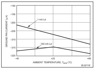
Figure 7. Ground pin current versus temperature.
