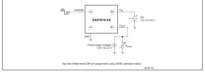
Figure 1. Simplified device diagram.
