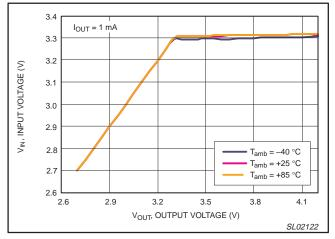
Figure 5. Input voltage versus output voltage.
