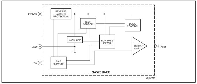
Figure 9. Simplified block diagram.
