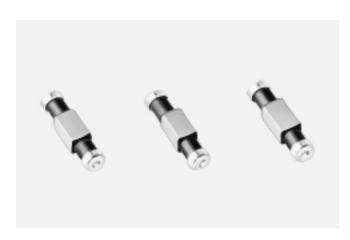
The T-type chip, NFM61R/RH, is a 3 terminal capacitor capable of carrying the large currents (2A) required for use in DC power circuits. This chip series consists of a T-type filter circuit incorporating a ferrite bead inductor for the purpose of suppressing undesirable oscillation. The heavy duty NFM61RH is an improved version of the filter for use in harsh operating conditions.
