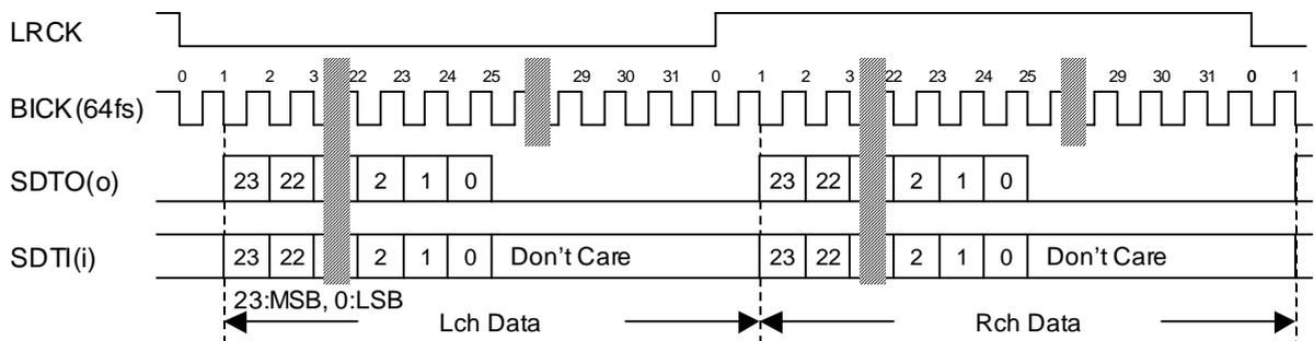
Figure 8. Audio Data Timing (SDTO: Mode1/3, SDTI: Mode3)
