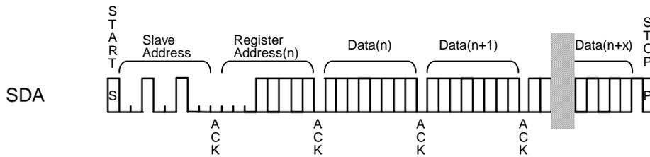
Figure 25. WRITE Operation
