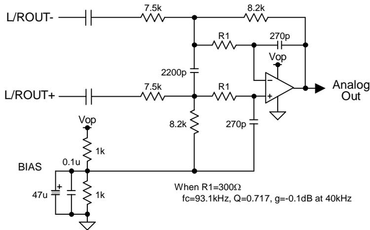
Figure 12. External 2<sup>nd</sup> order LPF Circuit Example (using op-amp with single power supply)
