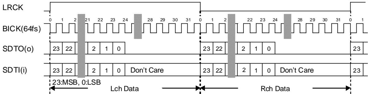
Figure 7. Audio Data Timing (SDTO: Mode0/2, SDTI: Mode2)
