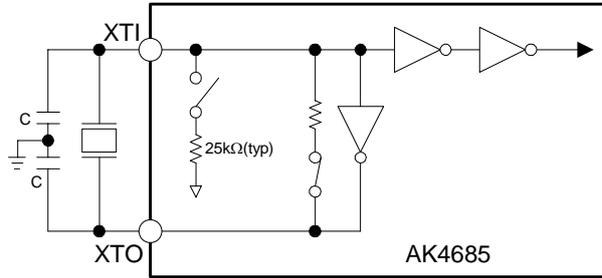
Note 29. The capacitor value is depend on the crystal oscillator (Typ.10-40pF)
