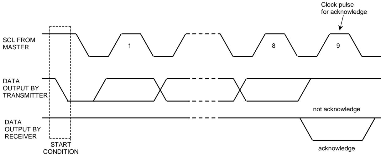
Figure 21. Acknowledge on the I<sup>2</sup>C-bus
