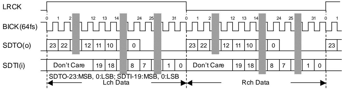
Figure 5. Audio Data Timing (SDTO: Mode0/2, SDTI: Mode0)
