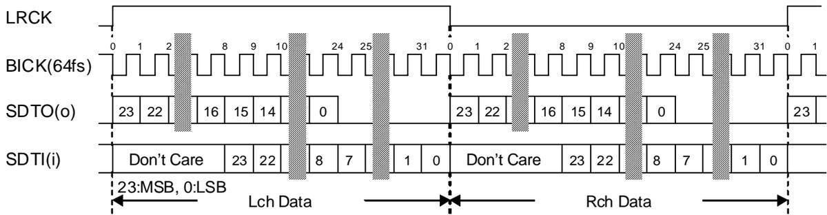
Figure 6. Audio Data Timing (SDTO: Mode0/2, SDTI: Mode1)
