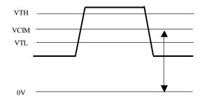
Figure : LVDS Differential Voltage
