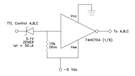
Control inputs A, B, and C can be driven directly with TTL logic with -5 Volts applied to the HCT logic gates Vee pin and to the Vee pad of the RF Switch.
