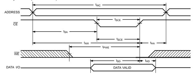
Write Cycle No. 2 (WE Controlled, OE HIGH During Write)<sup>[16, 17]</sup>
