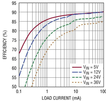
**Burst Mode Efficiency,  $V_{OUT} = 24\text{V}$ ,  $L = 15\mu\text{H}$**
