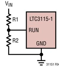
Figure 4. Setting the Input UVLO Threshold and Hysteresis
