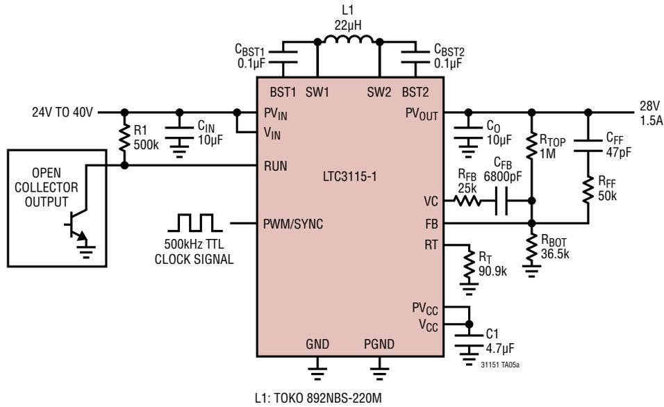
Output Voltage from Noisy Input Rail
