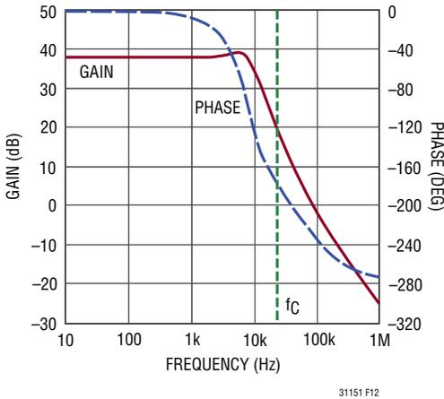
Figure 12. Converter Bode Plot,  $V_{IN} = 3.5V$ ,  $I_{LOAD} = 500mA$
