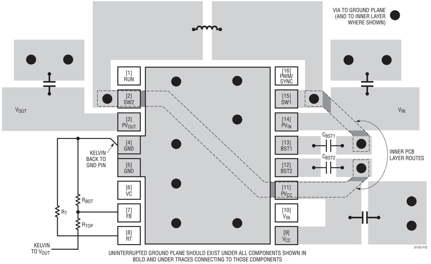
Figure 15. PCB Layout Recommended for the DHD Package
