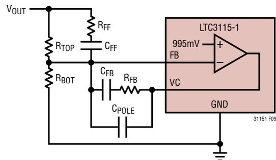
Figure 9. Error Amplifier with Type III Compensation
