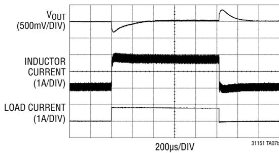
Transient Response to 800mA Load Step, V<sub>IN</sub> = 24V
