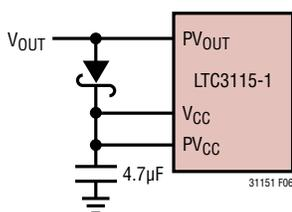
Figure 6. Bootstrapping PV<sub>CC</sub> and V<sub>CC</sub>
