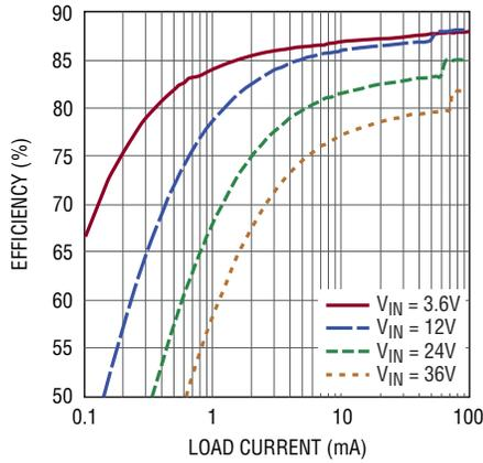
**Burst Mode Efficiency,  $V_{OUT} = 12\text{V}$ ,  $L = 15\mu\text{H}$**
