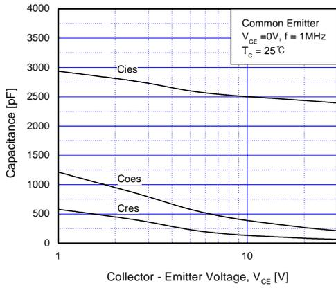
**Fig 7. Capacitance Characteristics**
