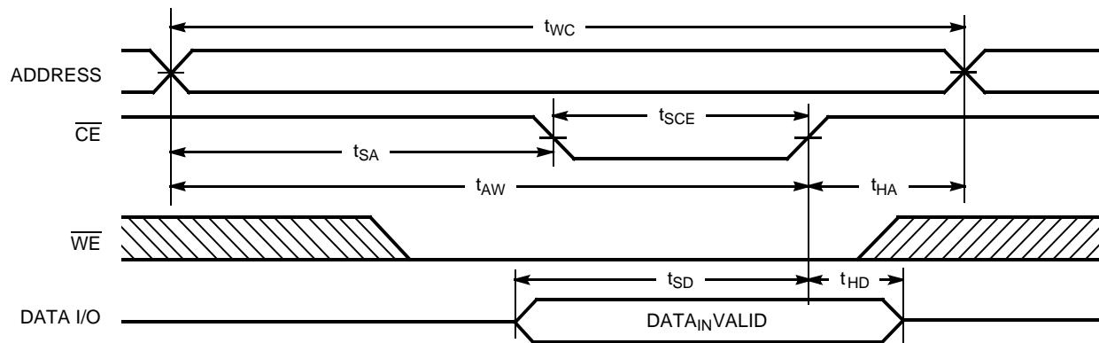
**Write Cycle No. 3 ( $\overline{WE}$  Controlled,  $\overline{OE}$  LOW)<sup>[11, 16]</sup>**
