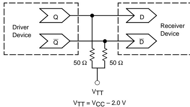
**Typical Termination for Output Driver and Device Evaluation**
