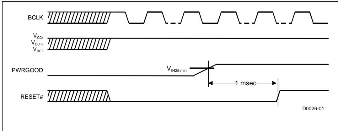
The PWRGOOD signal, which must be supplied to the processor, is used to protect internal circuits against voltage sequencing issues. The PWRGOOD signal should be driven high throughout boundary scan operation.
