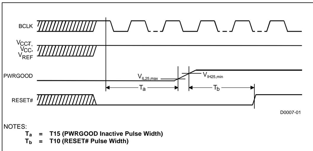
Figure 11. Test Timings (Boundary Scan)
