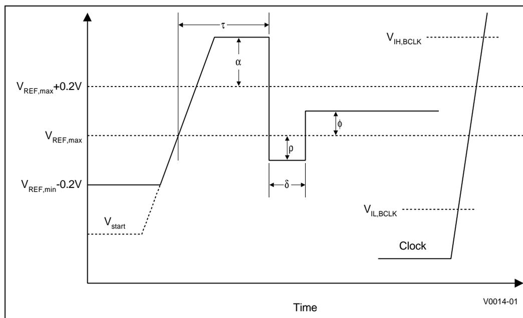
Figure 17. High to Low, GTL+ Receiver Ringback Tolerance
