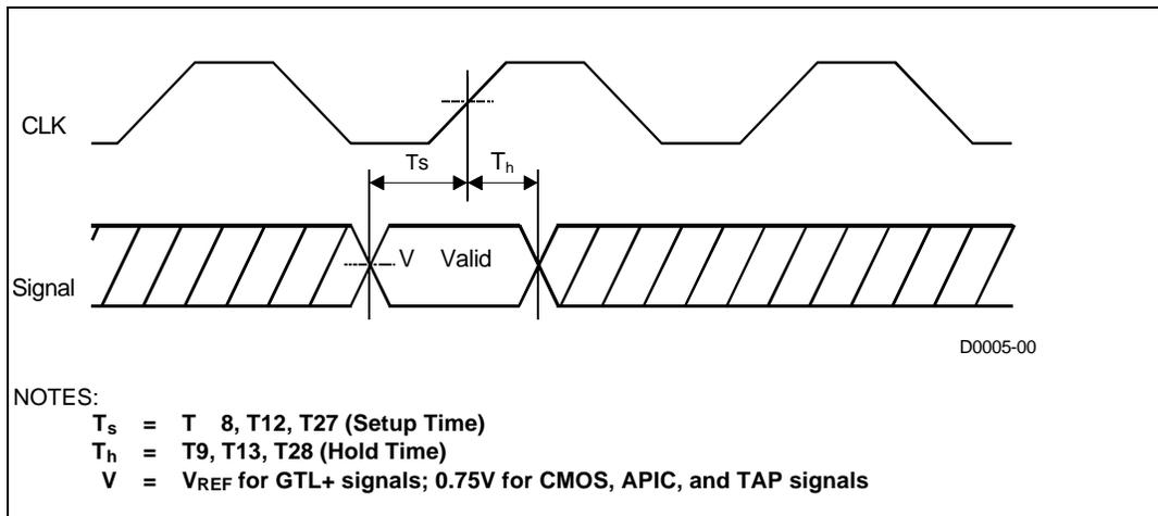
Figure 9. Cold/Warm Reset and Configuration Timings
