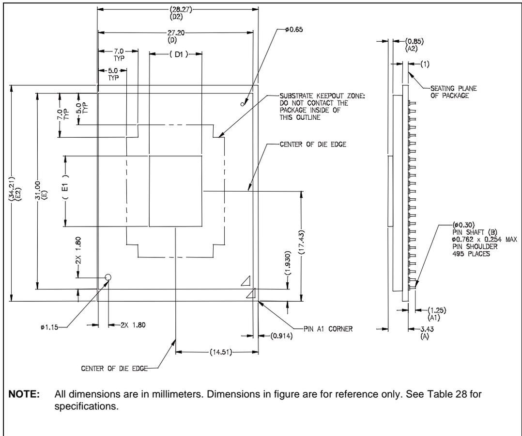
Figure 22. Socketable Micro-PGA2 Package - Bottom View
