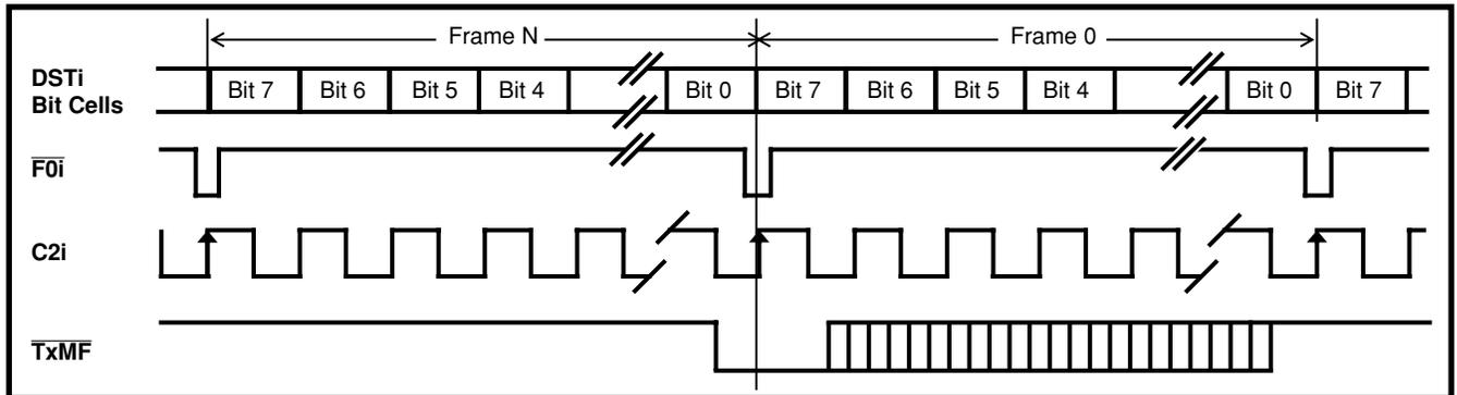
**Figure 20 - Functional Timing for Transmit Multiframe Clock**
