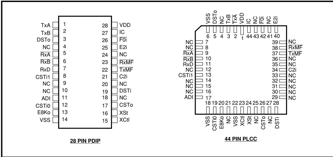
Figure 2 - Pin Connections
