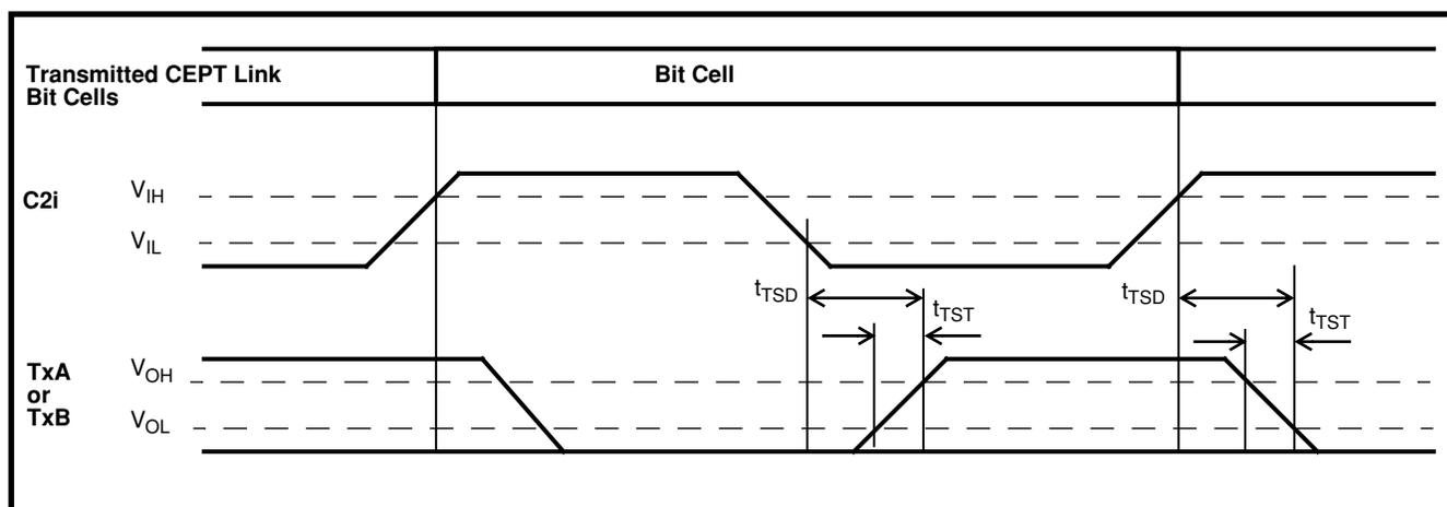
**Figure 25 - Transmit Timing for CEPT Link**
