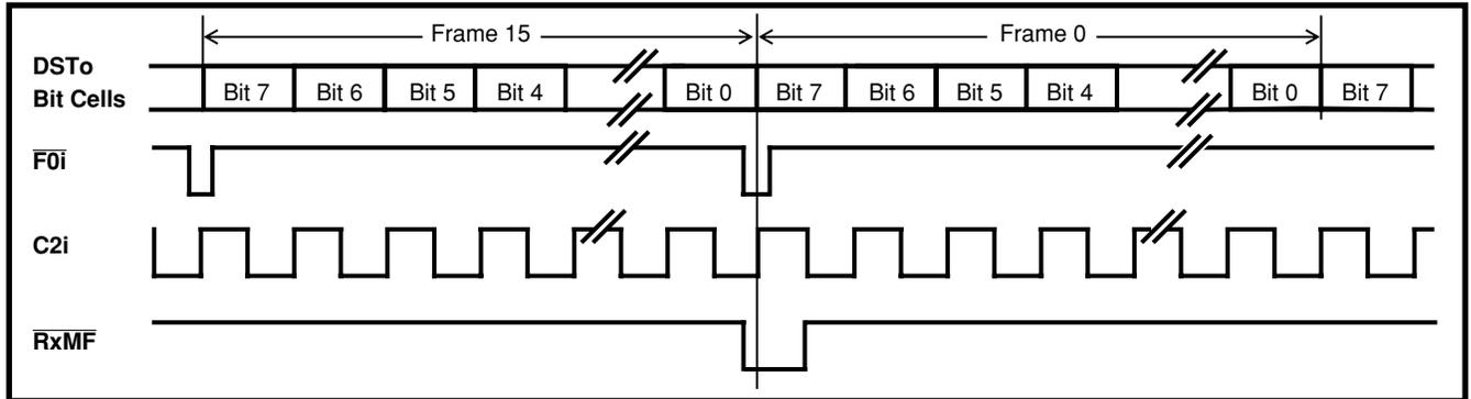
**Figure 19 - Functional Timing for Receive Multiframe Clocks**
