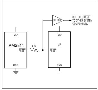
Figure 3. Interfacing to µPs with Bidirectional Reset I/O
