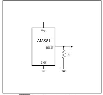
Figure 2.  $\overline{RESET}$  Valid to  $V_{CC}$  = Ground Circuit
