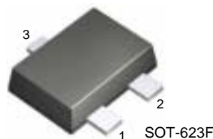
1. Base 2. Emitter 3. Collector
