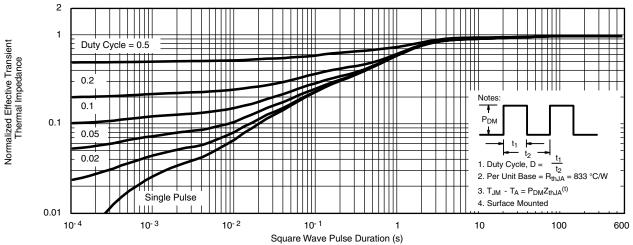
Normalized Thermal Transient Impedance, Junction-to-Ambient (SC-75A)
