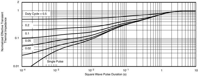
Normalized Thermal Transient Impedance, Junction-to-Foot
