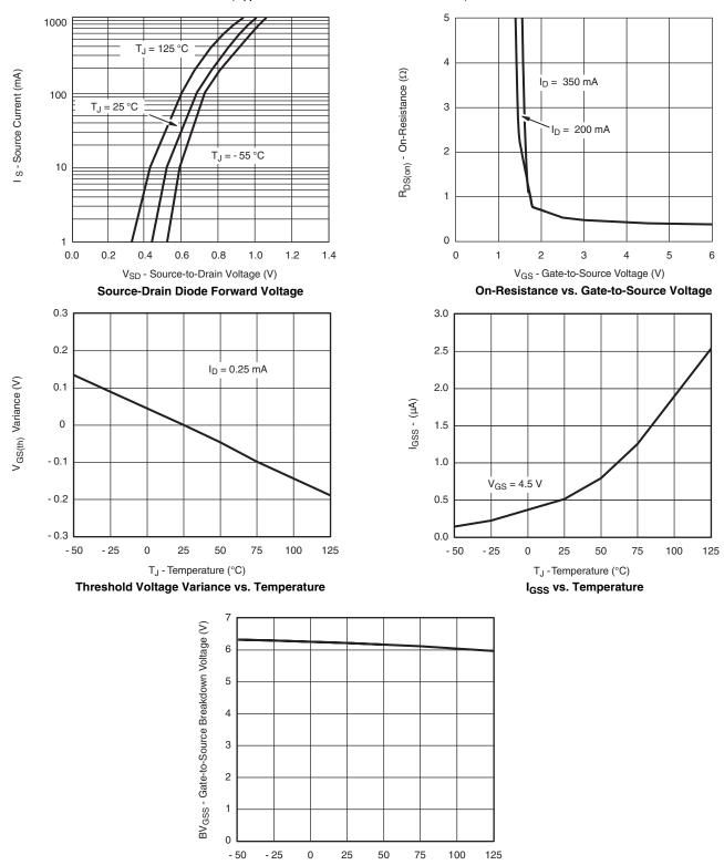
$T_J$  - Temperature (°C) BV<sub>GSS</sub> vs. Temperature
