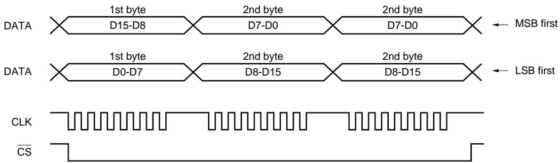
The 2-byte successive command writes characters to the video RAM. To successively write characters without changing the blinking data, reverse specification data, and Vc2 specification data, first transfer the first byte and then transfer the second byte (character address).
