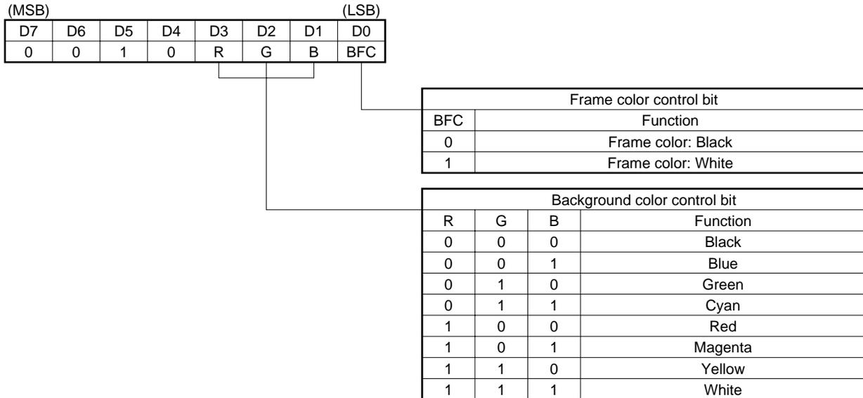
**(2) With LSB first (Use of each bit is the same as (1). The command is input from LSB (D0).)**
