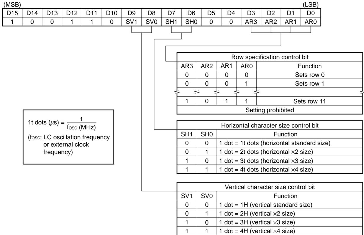
**(2) With LSB first (Use of each bit is the same as (1). The command is input from LSB (D0).)**
