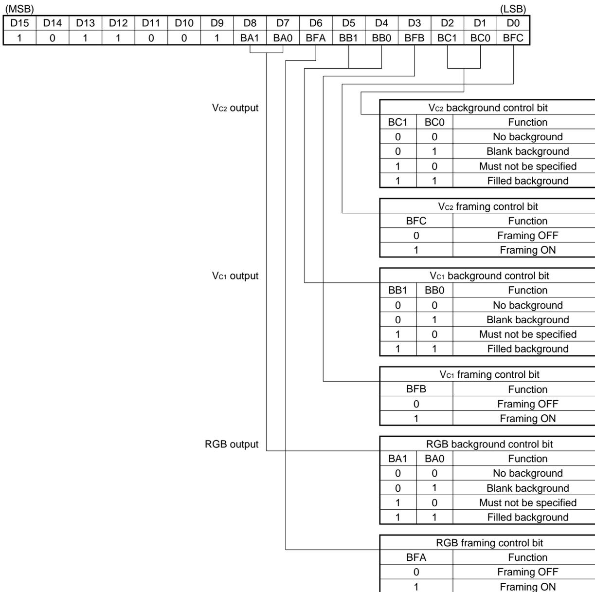
**(2) With LSB first (Use of each bit is the same as (1). The command is input from LSB (D0).)**
