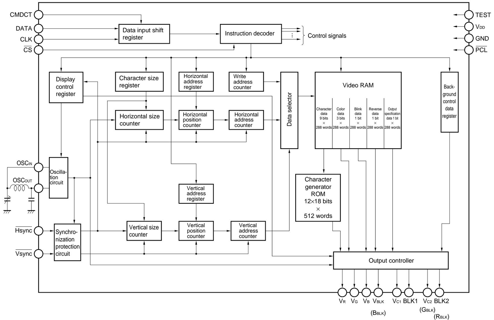
**Remark** Signals in ( ) are set by using an initial status setting command (RGB + RGB compatible blanking).
