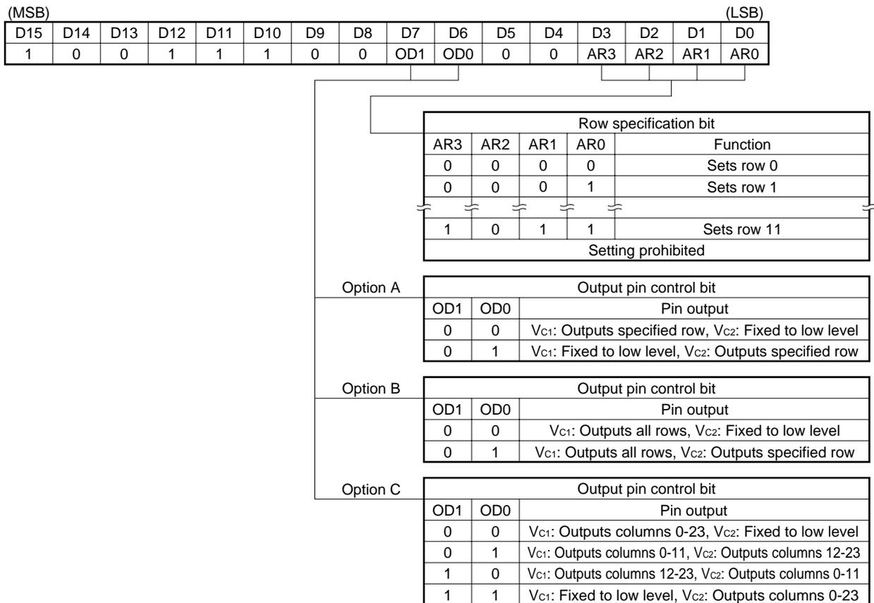
**(2) With LSB first (Use of each bit is the same as (1). The command is input from LSB (D0).)**
