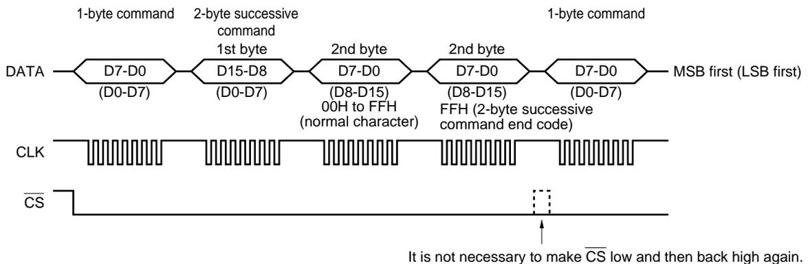
**Remark** By using the 2-byte successive command end code, the  $\overline{CS}$  pin may remain low. However, it is recommended to make  $\overline{CS}$  pin high to improve the noise immunity.
