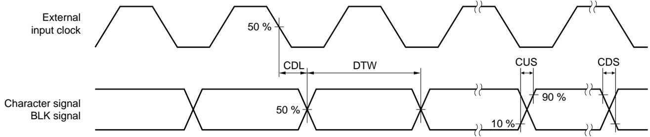
**Output Timing (T<sub>A</sub> = -20 to +75 °C, pins: V<sub>R</sub>, V<sub>G</sub>, V<sub>B</sub>, V<sub>BLK</sub>, V<sub>C1</sub>, BLK1, V<sub>C2</sub>, BLK2, (R<sub>BLK</sub>, G<sub>BLK</sub>, B<sub>BLK</sub>))**
