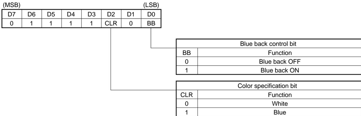
(2) With LSB first (Use of each bit is the same as (1). The command is input from LSB (D0).)
