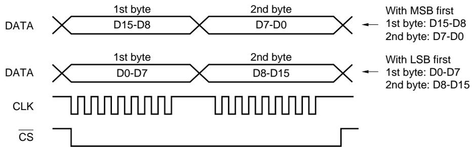
When transferring a 2-byte command, do not make  $\overline{CS}$  high and keep it low between the first and second bytes.
