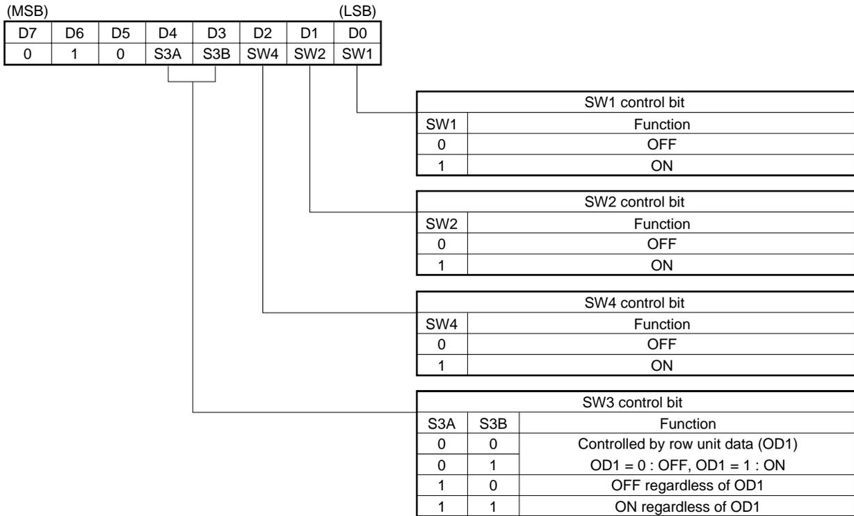
(2) With LSB first (Use of each bit is the same as (1). The command is input from LSB (D0).)
