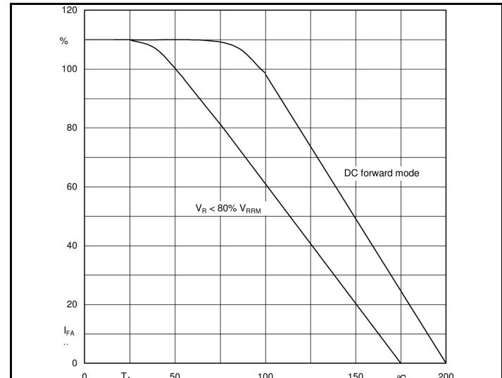
Fig. 2 Rated forward current vs. temp. of the terminals<sup>1)</sup>
