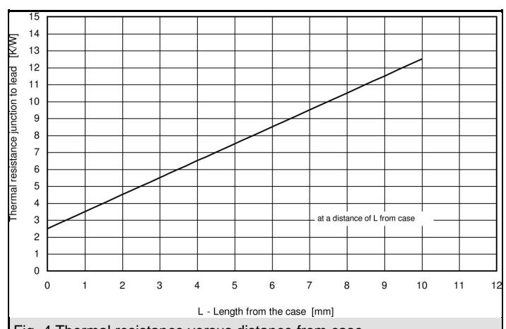
Fig. 4 Thermal resistance versus distance from case
