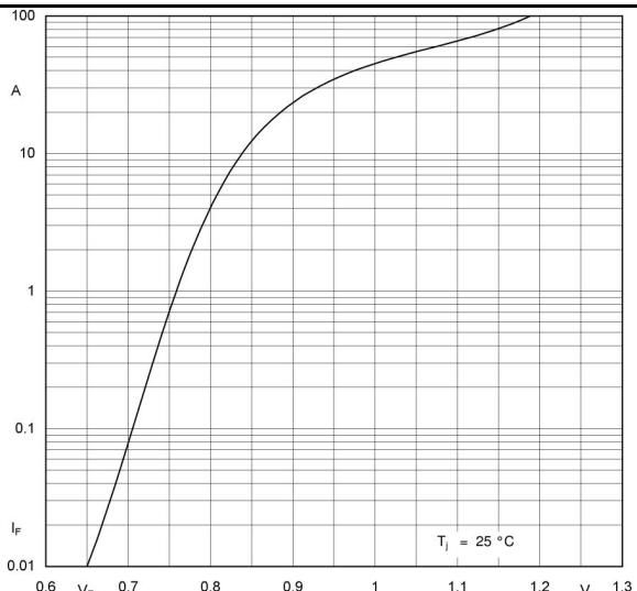
Fig. 1 Forward characteristic (typical value)<sup>1)</sup>
