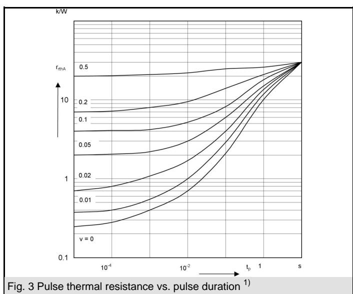
Fig. 3 Pulse thermal resistance vs. pulse duration<sup>1)</sup>
