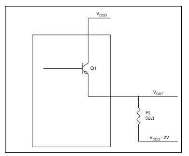
Figure 6. LVPECL Driver Circuit and Termination
