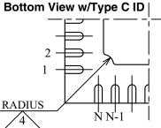
There are 2 methods of indicating pin 1 corner at the back of the VFQFN package are:
