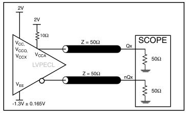
3.3V LVPECL Output Load AC Test Circuit
