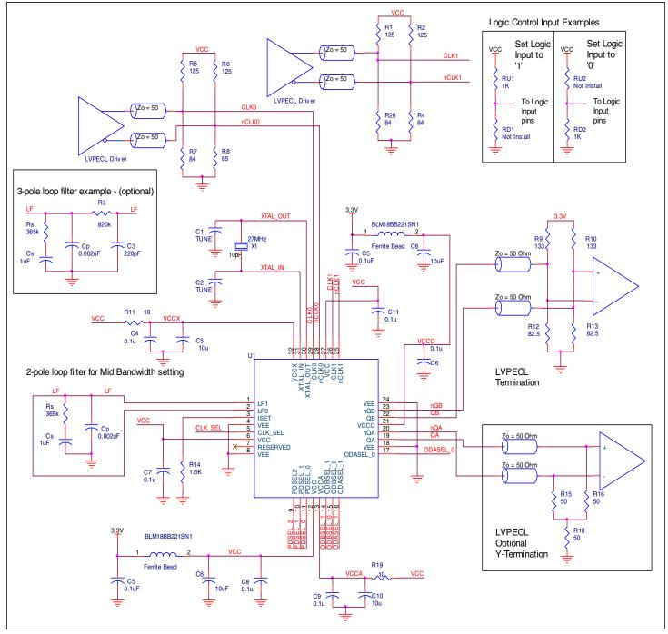
Figure 5. ICS813N252I-02 Schematic Example
