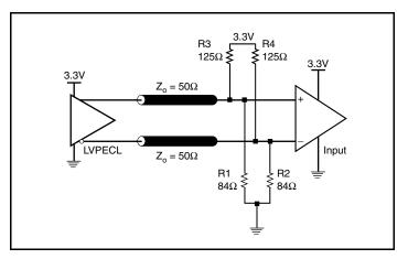
Figure 3B. 3.3V LVPECL Output Termination
