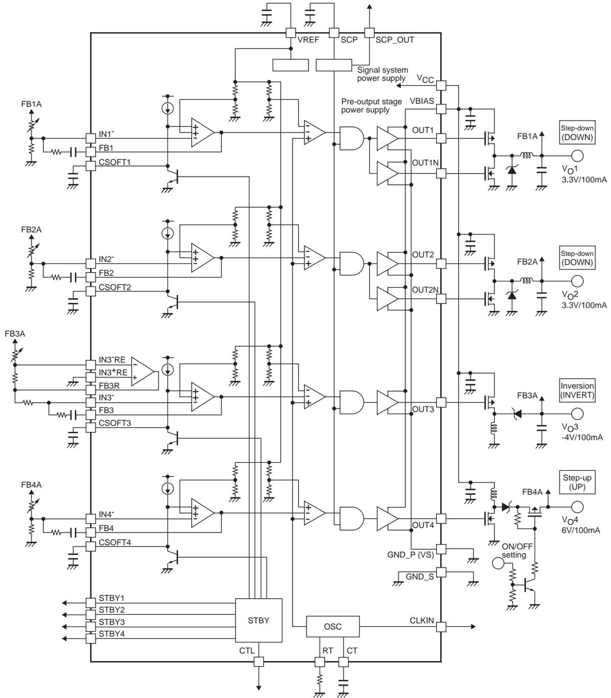
The CLKIN pin must be connected to GND, when the external clock synchronization (CLKIN) is not used.
