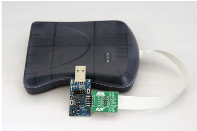
Figure 20. Connecting AVR JTAGICE mkII to the AT88Microbase
