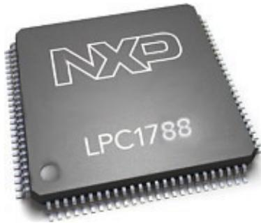
The NXP LPC1788 ARM Cortex-M3 based microcontroller runs the open source  $\mu$ EZ<sup>®</sup> + FreeRTOS software platform. The LPC1788 has 512KB of internal Flash memory, 96KB of internal SRAM, a 10/100 Ethernet Media Access Controller (MAC), a USB full speed device/host/OTG controller, four UARTs, two CAN channels and a collection of serial communications interfaces. The  $\mu$ EZ GUI board also includes 8MB of external SDRAM and 8MB of external NOR Flash.
