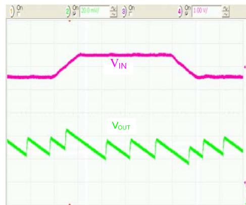
Figure 25. Line Transient Response in PFM Mode, 10 \mu s/div.
