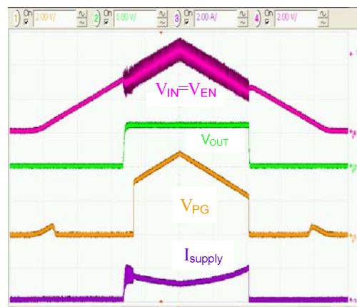
Figure 23. Soft-Start, EN Pin Tied to VCC R_{LOAD}=400m\Omega , C_{OUT}=100\mu F , 1ms/div.
