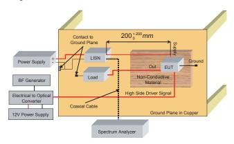
Figure 23. Test Bench for Conducted Emission
