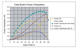
Figure 42. Total Board Power Dissipation
