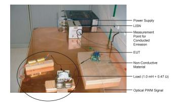
Figure 26. Conducted Emission Test Setup
