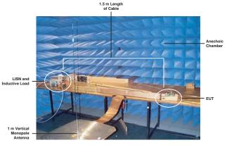
Figure 31. Radiated Emission Test Set Up
