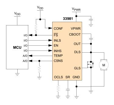
Figure 1. 33981 Simplified Application Diagram
