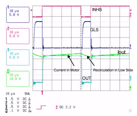
Figure 17. Cross-Conduction with Low Side
