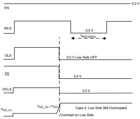
Figure 14. Overload on Low Side Gate Drive, Case 2
