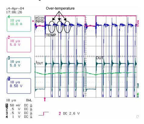
Figure 18. Over-temperature on OUT
