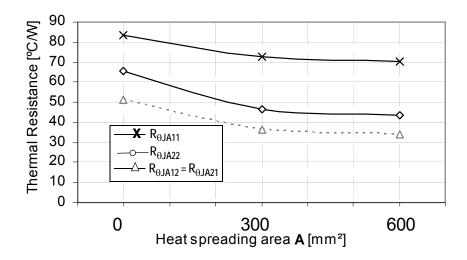
Figure 46. Device on Thermal Test Board  $R_{\theta J A}$
