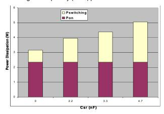
Figure 41. Power Switching vs. SR Capacitor
