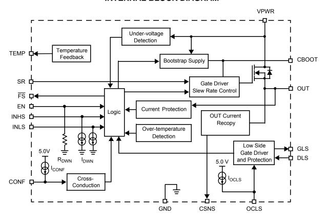
Figure 2. 33981 Simplified Internal Block Diagram
