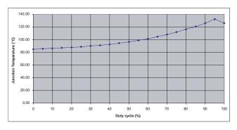
Figure 43. Junction Temperature vs. Duty Cycle
