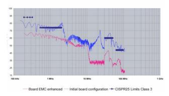
Figure 30. Conducted Emission Spectrum for 33981
