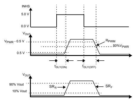
Figure 4. Time Delays Functional Diagrams
