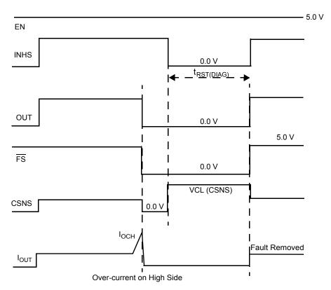
Figure 15. Over-current on Output
