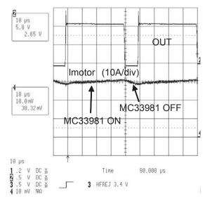
Figure 34. Current and Voltage waveforms
