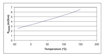
Figure 35. R<sub>DS(ON)</sub> vs. Temperature
