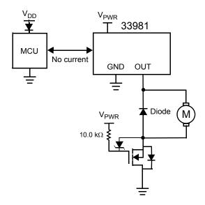
Figure 11. Reverse Battery Protection
