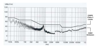
Figure 32. Radiated Emission Spectrum for 33981
