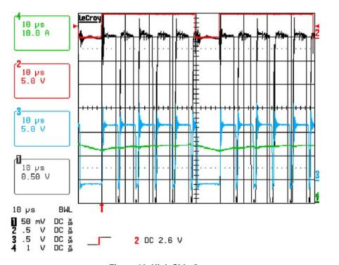
Figure 16. High Side Over-current
