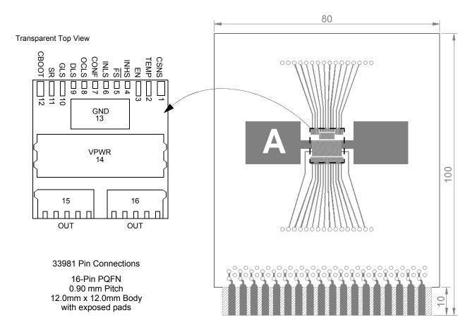
Figure 45. Thermal Test Board
