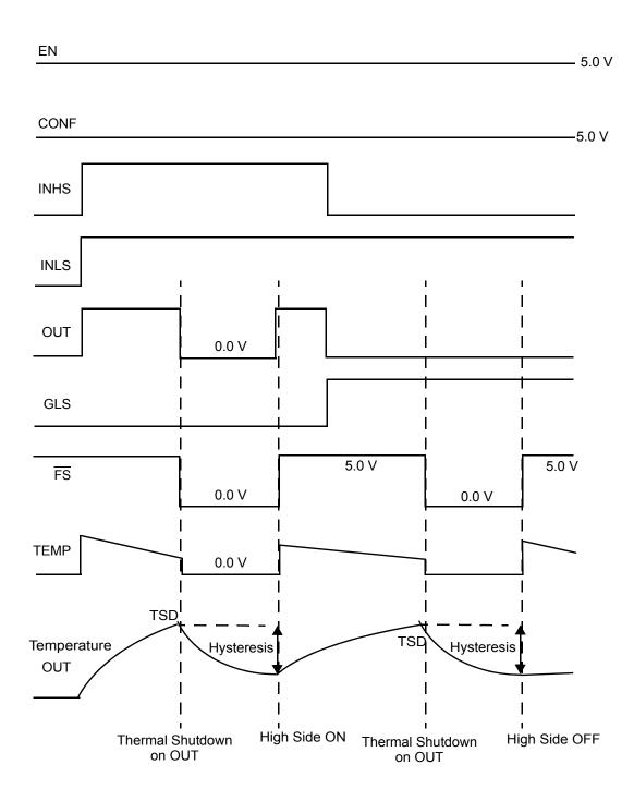
Figure 12. Over-temperature on Output
