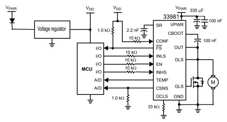
Figure 20. 33981 Typical Application Diagram
