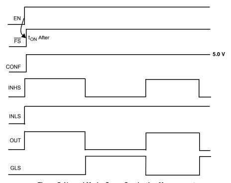
Figure 5. Normal Mode, Cross-Conduction Management
