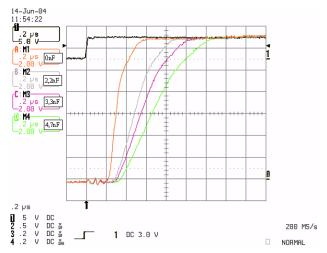
Figure 37. OUT switching vs. SR Capacitor
