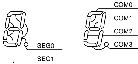
Figure 23-6 Example of COM and SEG Pin Connections (1/4 Duty)
