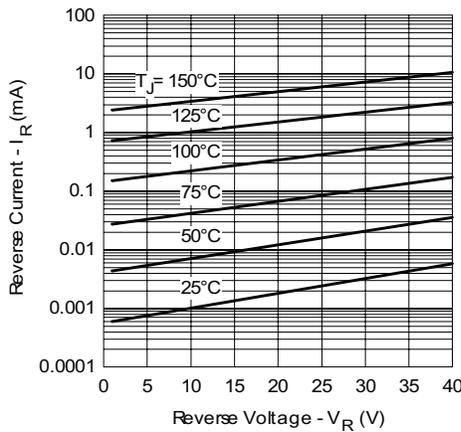
Fig. 2 - Typical Peak Reverse Current vs. Reverse Voltage
