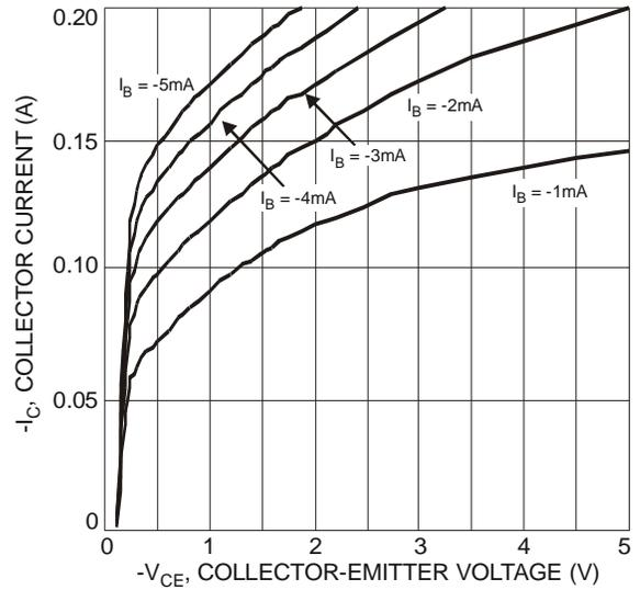
Fig. 2 Typical Collector Current vs. Collector-Emitter Voltage (DN0150BLP4)
