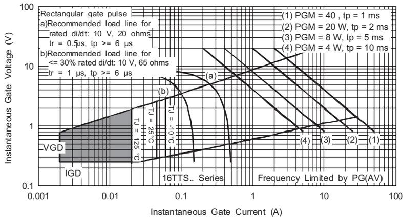
Fig. 9 - Gate Characteristics
