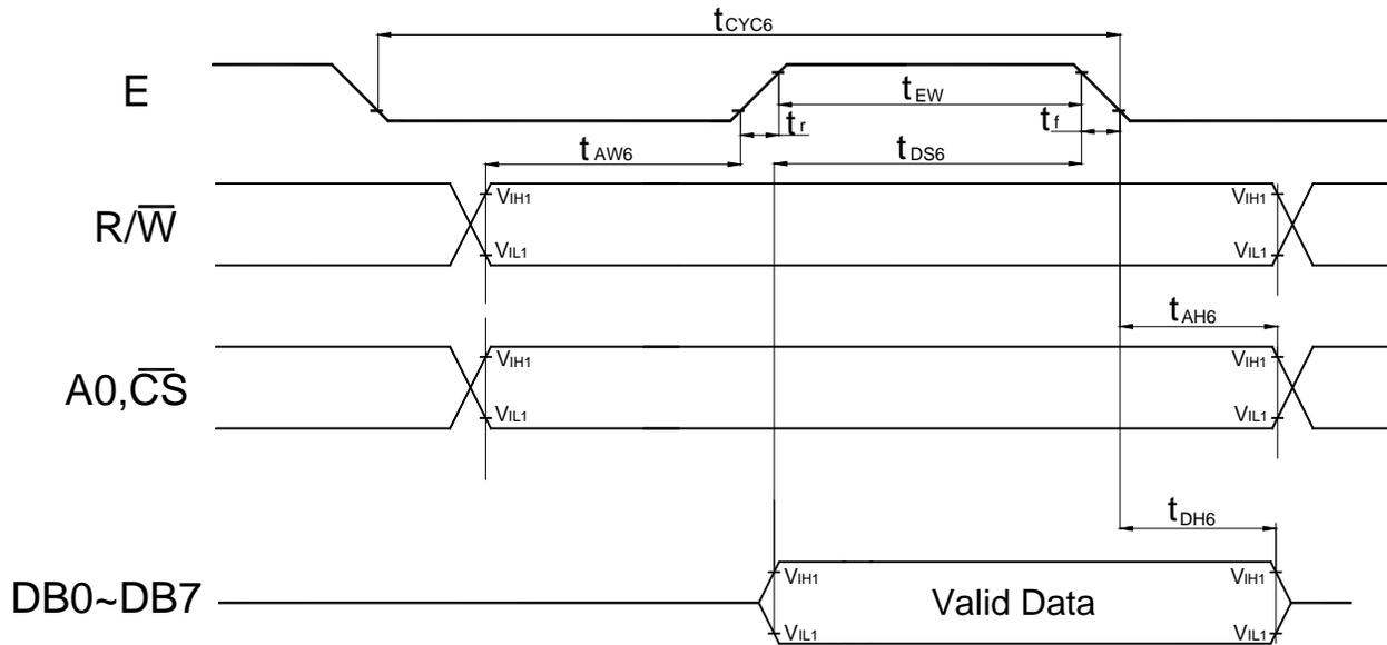
Fig. b Interface timing (data Write)
