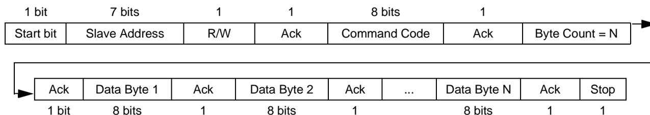
**Figure 9. An Example of a Block Write<sup>[8]</sup>**
