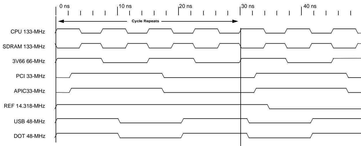
**Figure 5. Group Offset Waveforms (133-MHz CPU/133-MHz SDRAM Clock)**
