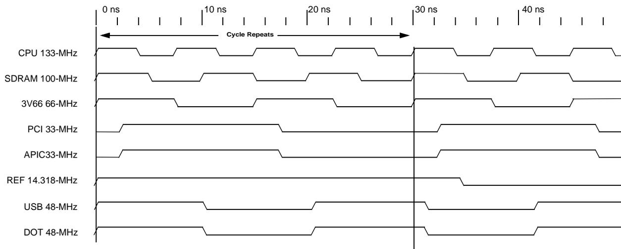
**Figure 4. Group Offset Waveforms (133-MHz CPU/100-MHz SDRAM Clock)**
