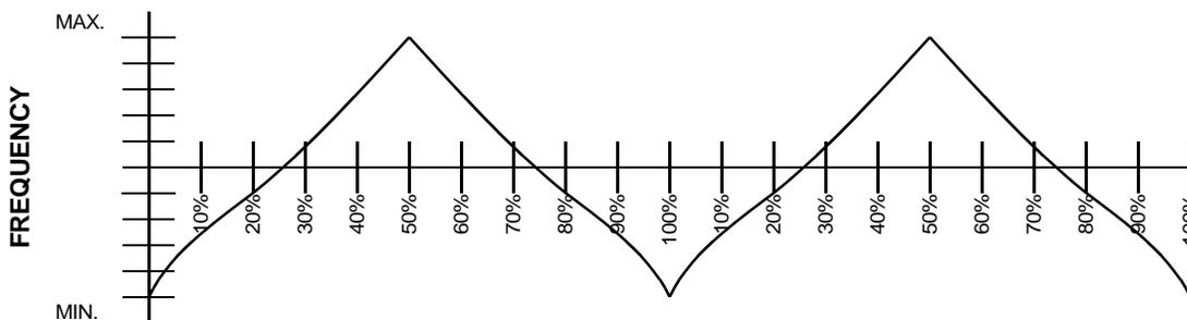
Figure 8. Typical Modulation Profile
