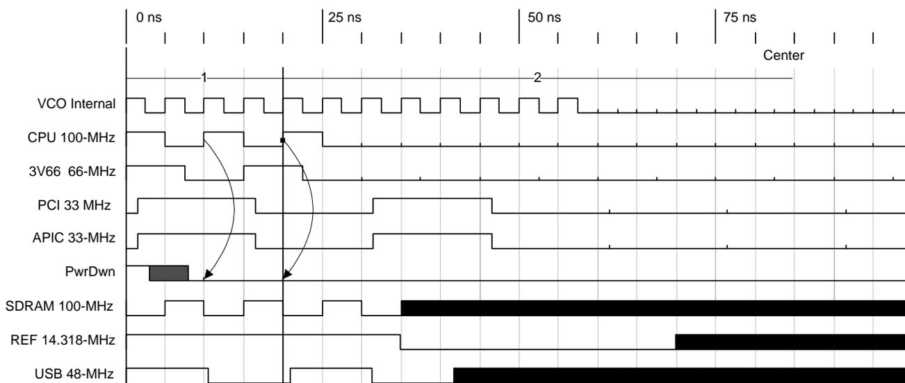
**Figure 6. W254B PWR\_DWN# Timing Diagram**<sup>[4, 5, 6, 7]</sup>
