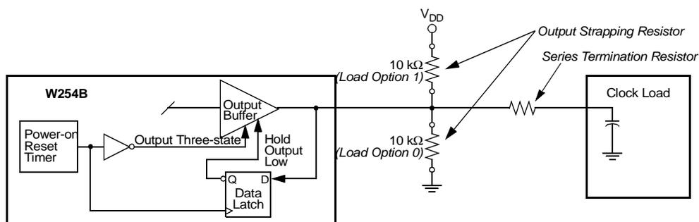
**Figure 1. Input Logic Selection Through Resistor Load Option**
