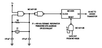
Figure 17. Using a Ceramic Resonator to Generate Carrier Frequency
