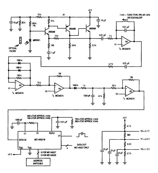
Figure 18. Infrared Receiver
