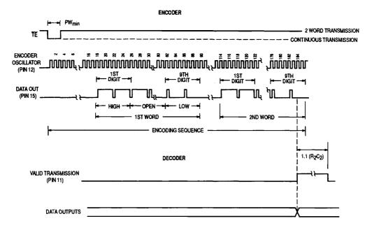
Figure 10. Timing Diagram
