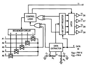
Figure 2. MC145027 Decoder Block Diagram
