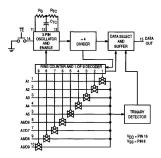
Figure 1. MC145026 Encoder Block Diagram
