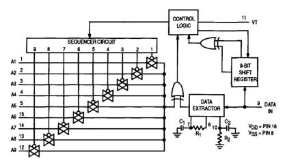
Figure 3. MC145028 Decoder Block Diagram
