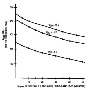
Figure 14. f<sub>max</sub> vs C<sub>layout</sub> — Decoders Only
