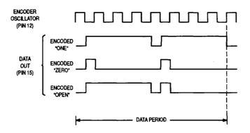
Figure 11. Encoder Data Waveforms
