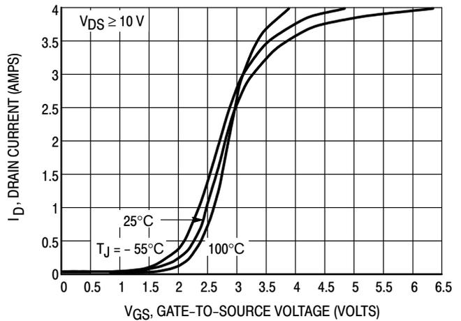
Figure 2. Transfer Characteristics
