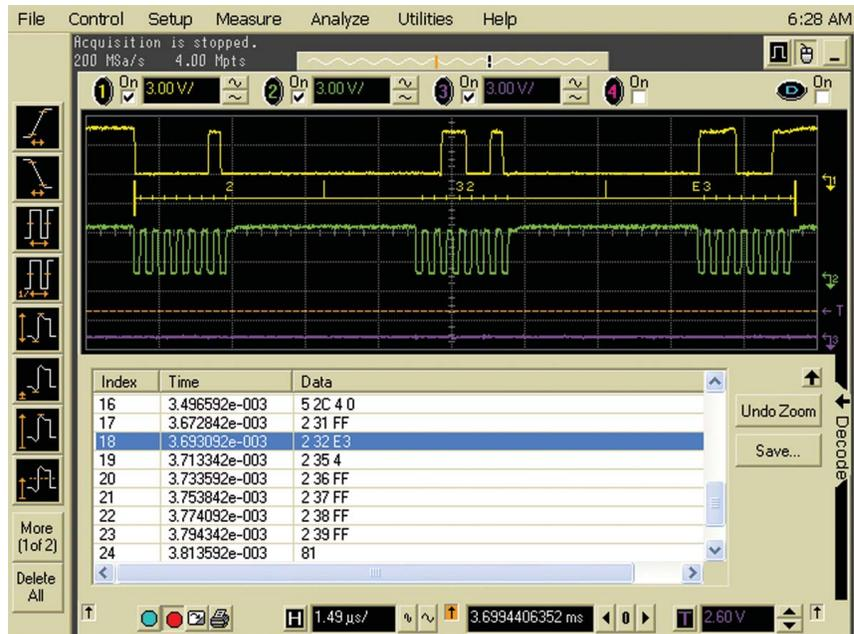
**Figure 9:** Listing window of a SPI capture, demonstrating the automatic click and zoom capability. The item in the listing window that was clicked on becomes highlighted in blue. After clicking on an item, the Undo Zoom button becomes available in the listing window.
