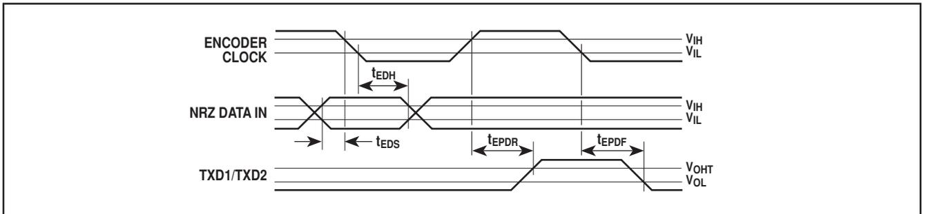
Figure 9 - Encoder timing parameters
