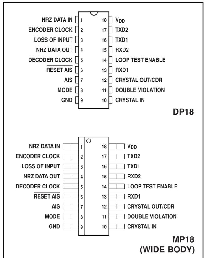
Figure 1 - Pin connections – top view
