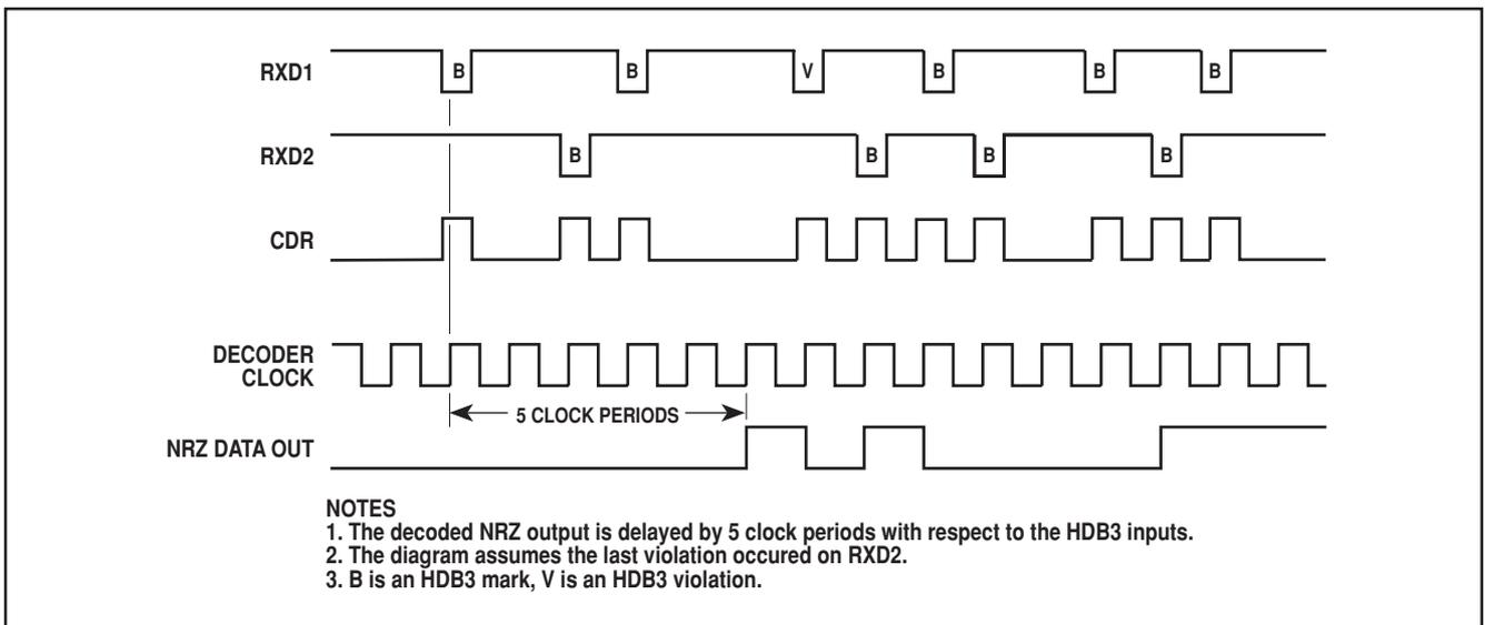
Figure 4 - Decoder waveforms
