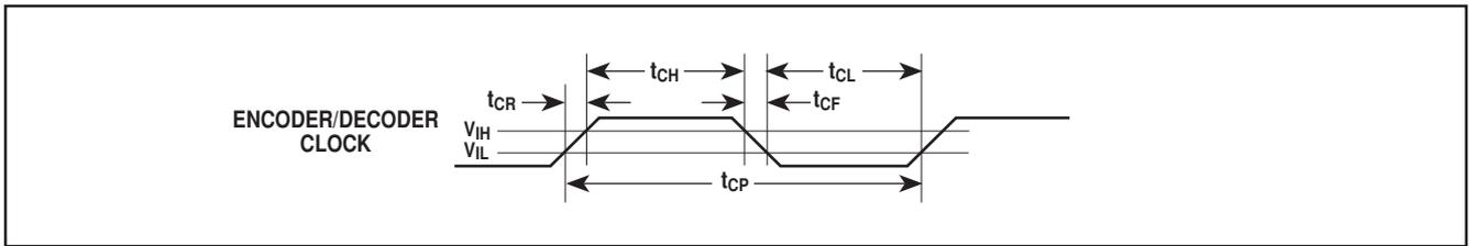
Figure 8 - Clock timing parameters
