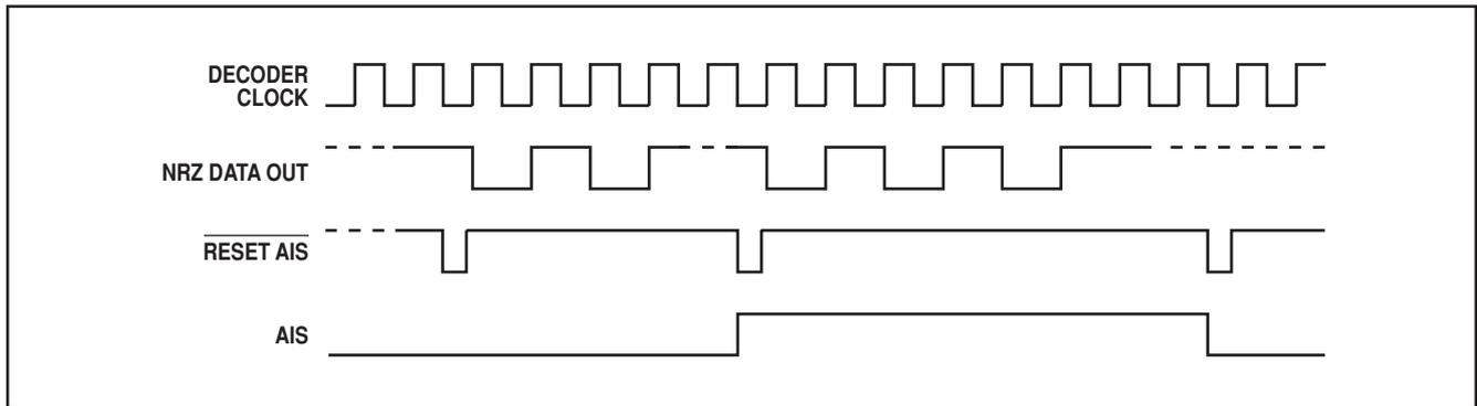
Figure 7 - AIS and  $\overline{\text{RESET AIS}}$  waveforms
