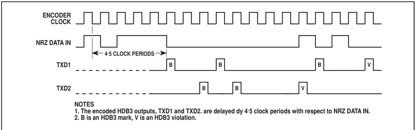
Figure 3 - Encoder waveforms
