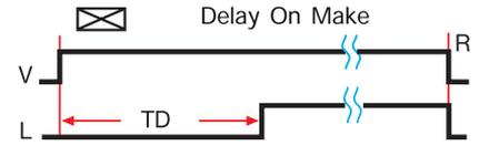
V = Voltage R = Reset TD = Time Delay
