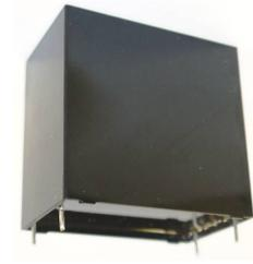
Non-inductive construction using metallized polypropylene film with flame retardant epoxy resin and case.
