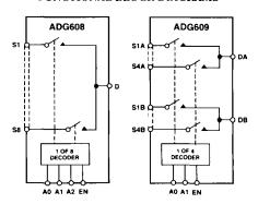
The ability to operate from single +3 V, +5 V or ±5 V bipolar supplies makes the ADG608 and ADG609 perfect for use in battery operated instruments and with the new generation of DACs and ADCs from Analog Devices. The use of 5 V supplies and reduced operating currents gives much lower power dissipation than devices operating from ±15 V supplies.
