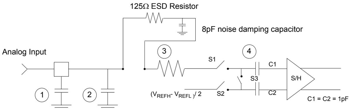
1. Parasitic capacitance due to package, pin-to-pin and pin-to-package base coupling; 1.8pF
