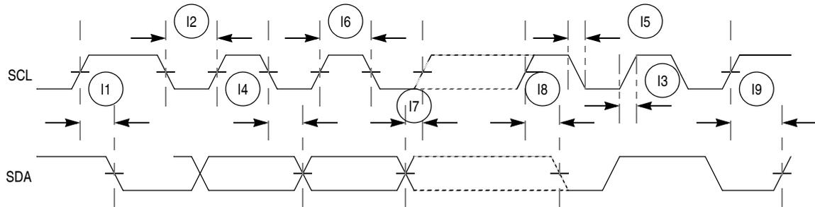
Figure 7. I<sup>2</sup>C Input/Output Timings
