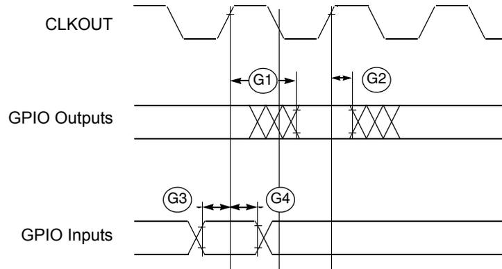
Figure 5. GPIO Timing
