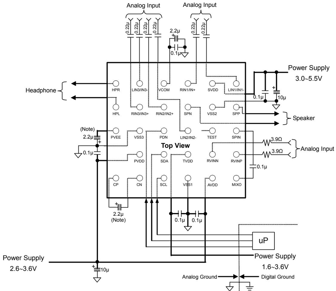
Figure 29. Typical Connection Diagram
