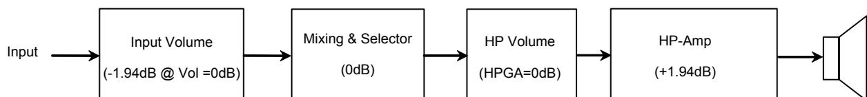
Figure 15. Headphone-Amp Path Level Diagram
