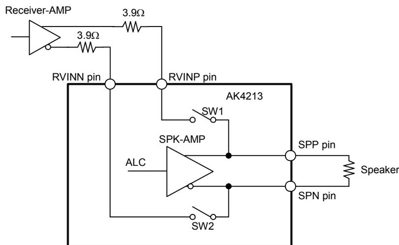
Figure 12. Bypass Mode
