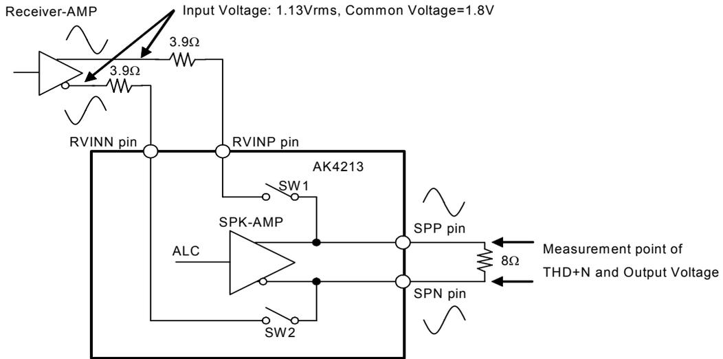
Figure 2. Connection with external RCV-Amp
