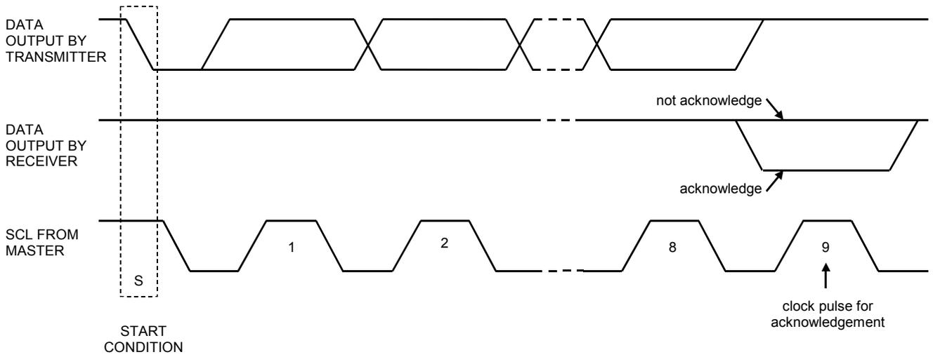
Figure 27. Acknowledge on the I<sup>2</sup>C-Bus
