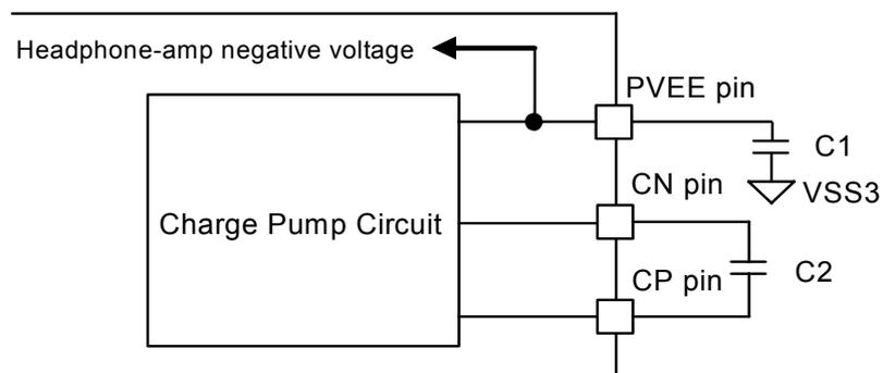
Figure 4. Charge Pump Circuit External Capacitor
