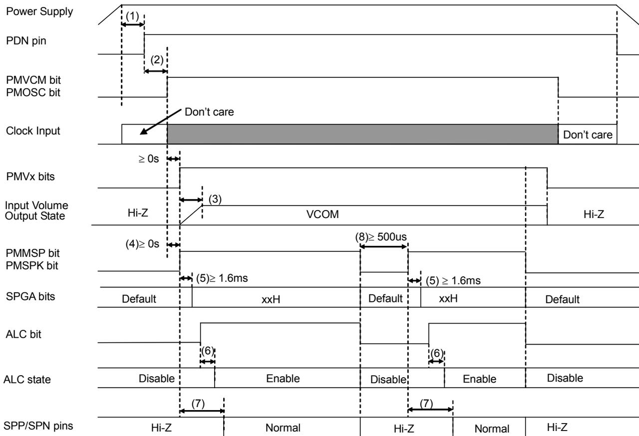
Figure 18. SPK-Amp Power-up/down Sequence Example
