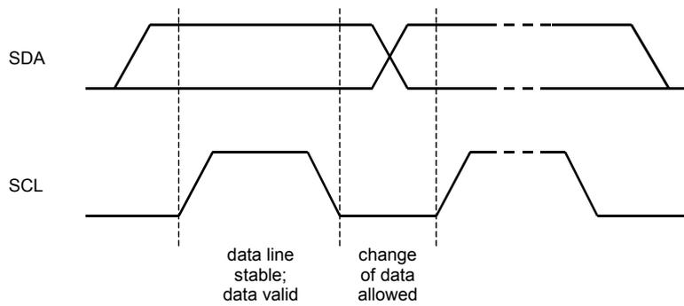
Figure 28. Bit Transfer on the I<sup>2</sup>C-Bus
