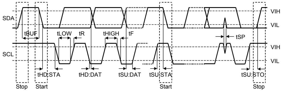
Figure 5. I<sup>2</sup>C Bus Mode Timing
