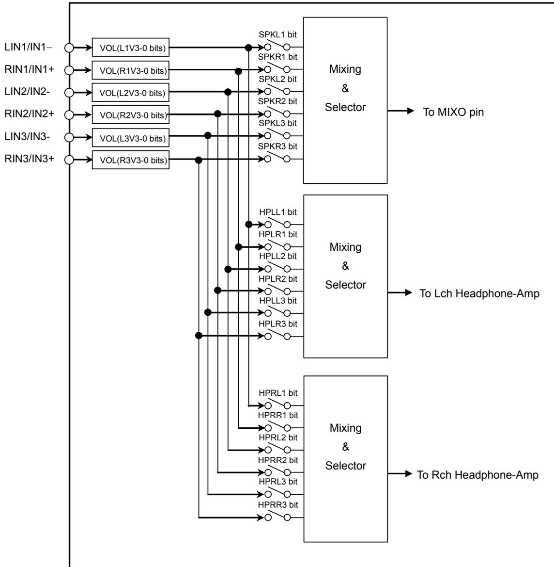
Figure 7. Input Selector & Volume in Single-ended Mode (SD3-1 bits = "000")
