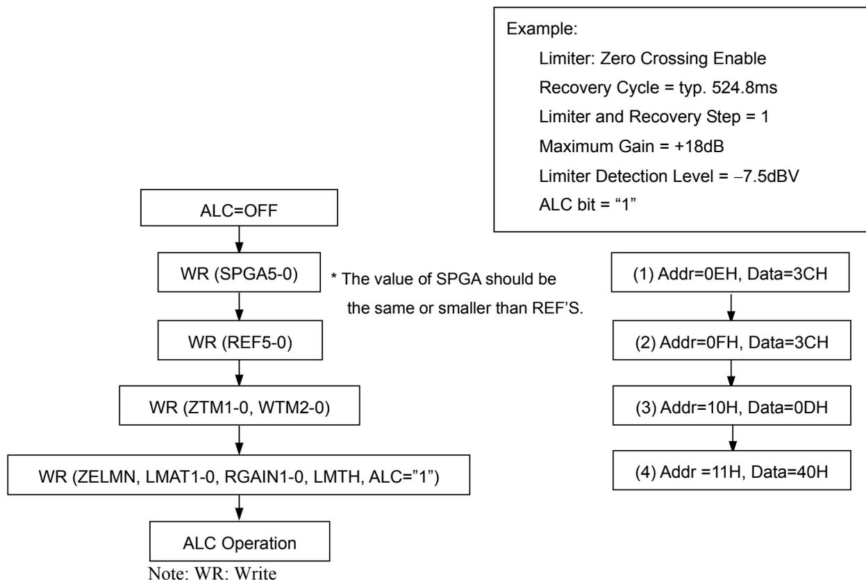
Figure 13. Registers set-up sequence at ALC operation
