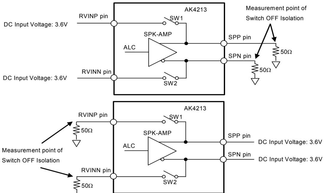
Figure 3. Measurement Circuit of Switch OFF Isolation
