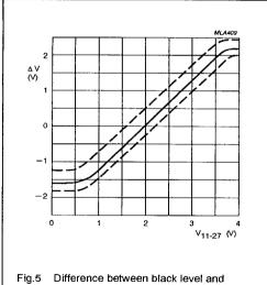
measuring level at the RGB outputs ( $\Delta V$ ) as a function of the brightness control input
